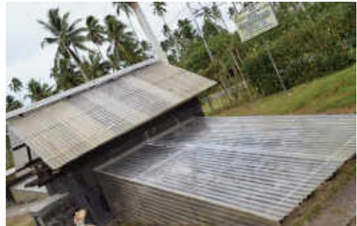
New Innovation: CCIL Combination Dryer, both Sun and hot air unit. The Combination drier is to be used by Partnership smallholder cooperatives to reduce 'smoke taint' contamination of dry beans. Important to maintain high quality of PNG Export Cocoa.
